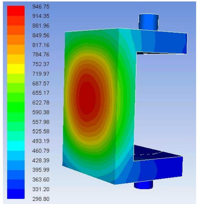
Figure 11a. Temperature contour of the Flat Plate surface with an incident flux of  $15 \text{ W/cm}^2$ .
