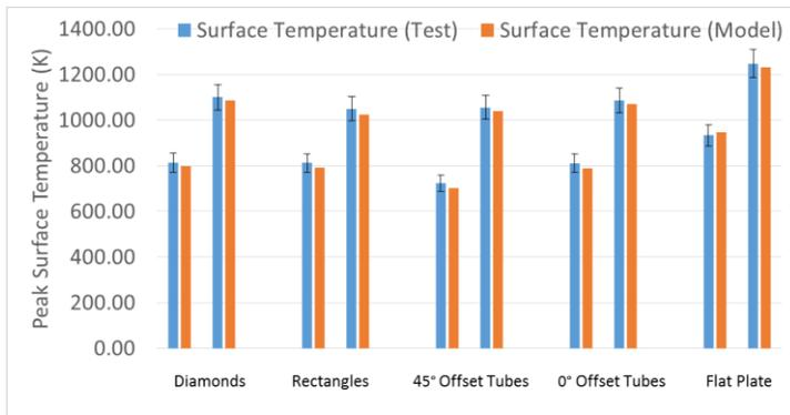
**Figure 14. Measured and simulated peak surface temperatures during tests of FLGs. Error bars represent the standard deviation on the measurements.**
