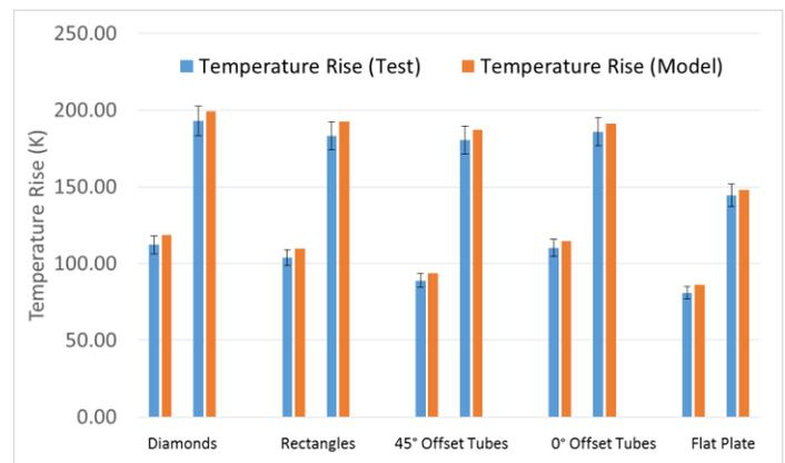
**Figure 13.** Measured and simulated air-temperature rise during tests of FLGs. Error bars represent the standard deviation on the measurements.
