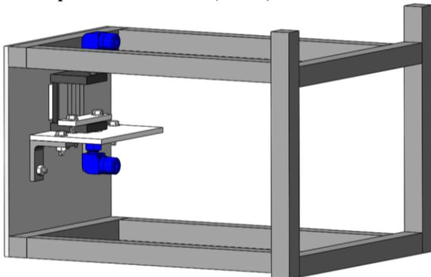
Figure 7. FLG complete mount. The part is located ~1.5 mm behind the 6.35 mm spillage board.
