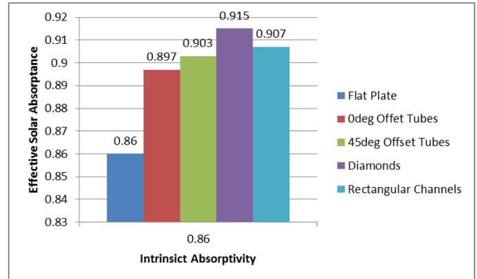
**Figure 3. Results of the ray-tracing simulations showing absorptance improvements from the fractal-like geometries relative to a flat plate receiver.**
