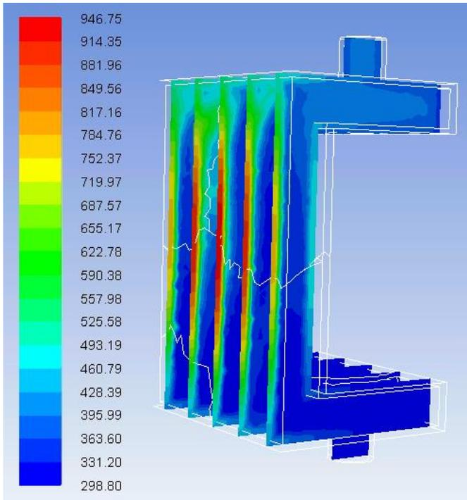
**Figure 11b.** Temperature contours of the air flow across the Flat Plate with an incident flux of  $15 \text{ W/cm}^2$ . Five cross-sectional planes with one centimeter separation.
