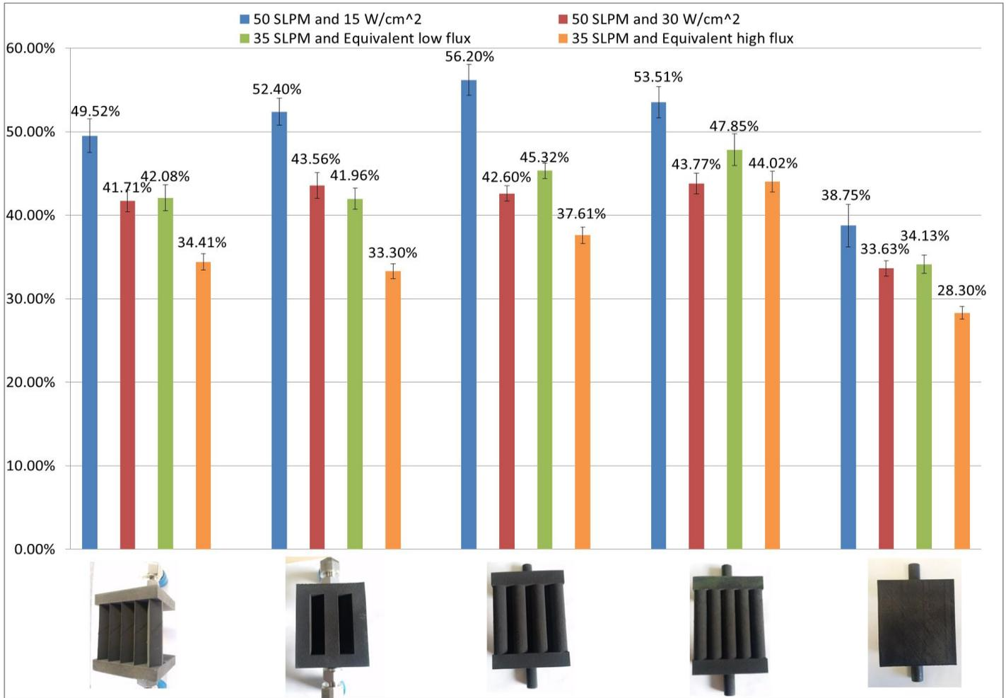
Figure 9. Thermal efficiency of FLGs. The equivalent high and low fluxes were estimated to match the outlet temperature of the 30 W/cm<sup>2</sup> and 15 W/cm<sup>2</sup> tests, respectively.
