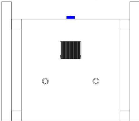
Figure 6. Spillage board located in the front of FLG mount. Aperture dimensions (W x L): 5 cm x 5.1 cm.
