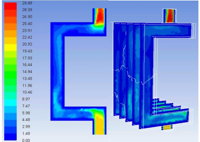
Figure 10. Velocity contours of the air flow across the Flat Plate. Left: Central cross-sectional plane. Right: Five cross-sectional planes with one centimeter separation.
