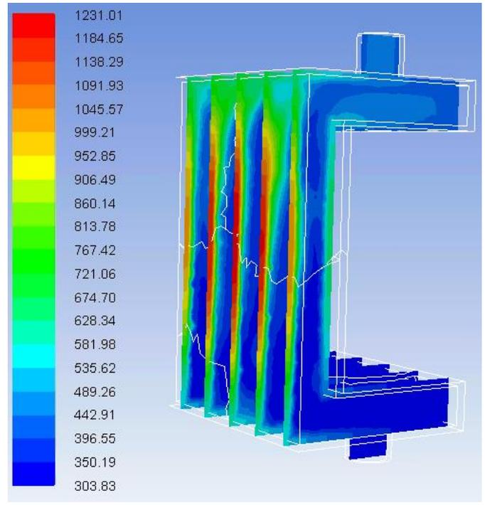
**Figure 12b.** Temperature contours of the air flow across the Flat Plate with an incident flux of  $30 \text{ W/cm}^2$ . Five cross-sectional planes with one centimeter separation.
