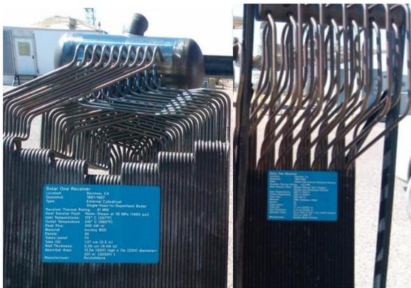
**Figure 1. Left: Solar One receiver panel. Right: Solar Two receiver panel.**
