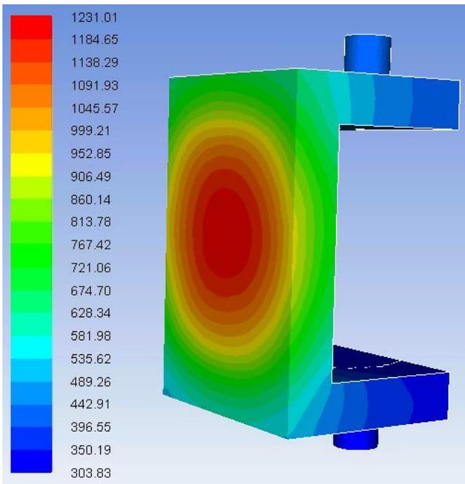
**Figure 12a.** Temperature contour of the Flat Plate surface with an incident flux of  $30 \text{ W/cm}^2$ .
