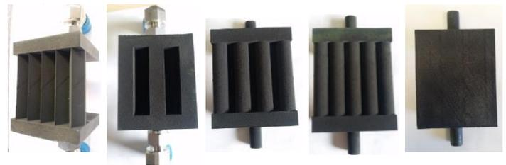
**Figure 4. New FLGs with manifolds manufactured by Sigma Labs (Santa Fe, NM). From left to right: diamond channels, rectangular channels, 45° offset cylinder tubes, 0° offset cylinder tubes, and flat plate [5].**
