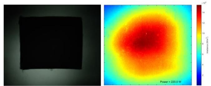
Figure 8a. Left: Heat flux incident on the flat plate. Right: Heat flux applied on the FLGs  $\sim 15 \text{ W/cm}^2$ .
