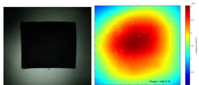
Figure 8b. Left: Heat flux incident on the flat plate. Right: Heat flux applied on the FLGs  $\sim 30 \text{ W/cm}^2$ .
